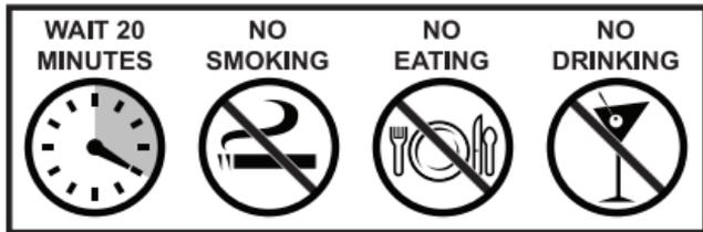
Wait 20 minutes after the test subject smokes, eats or drinks before testing. Failure to wait 20 minutes can give inaccurate BAC readings and damage the sensor.
